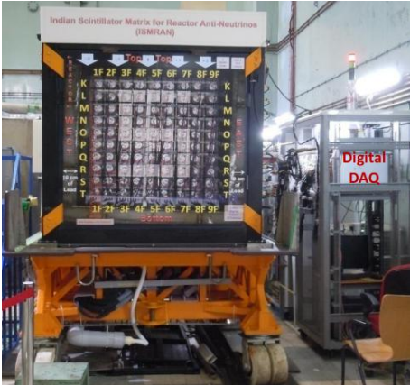
ISMARAN installed at 100MW Dhruva reactor (India), 2D segmented, plastic scintillator
