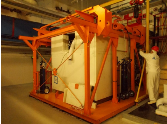
iDREAM has been installed and commissioned in 2021 at Kalinin NPP (Russia), 20m from 3GW reactor core, single volume, liquid scintillator
