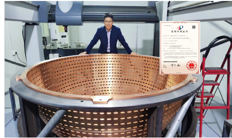
Uncovered half of the Copper Shell (CS)
