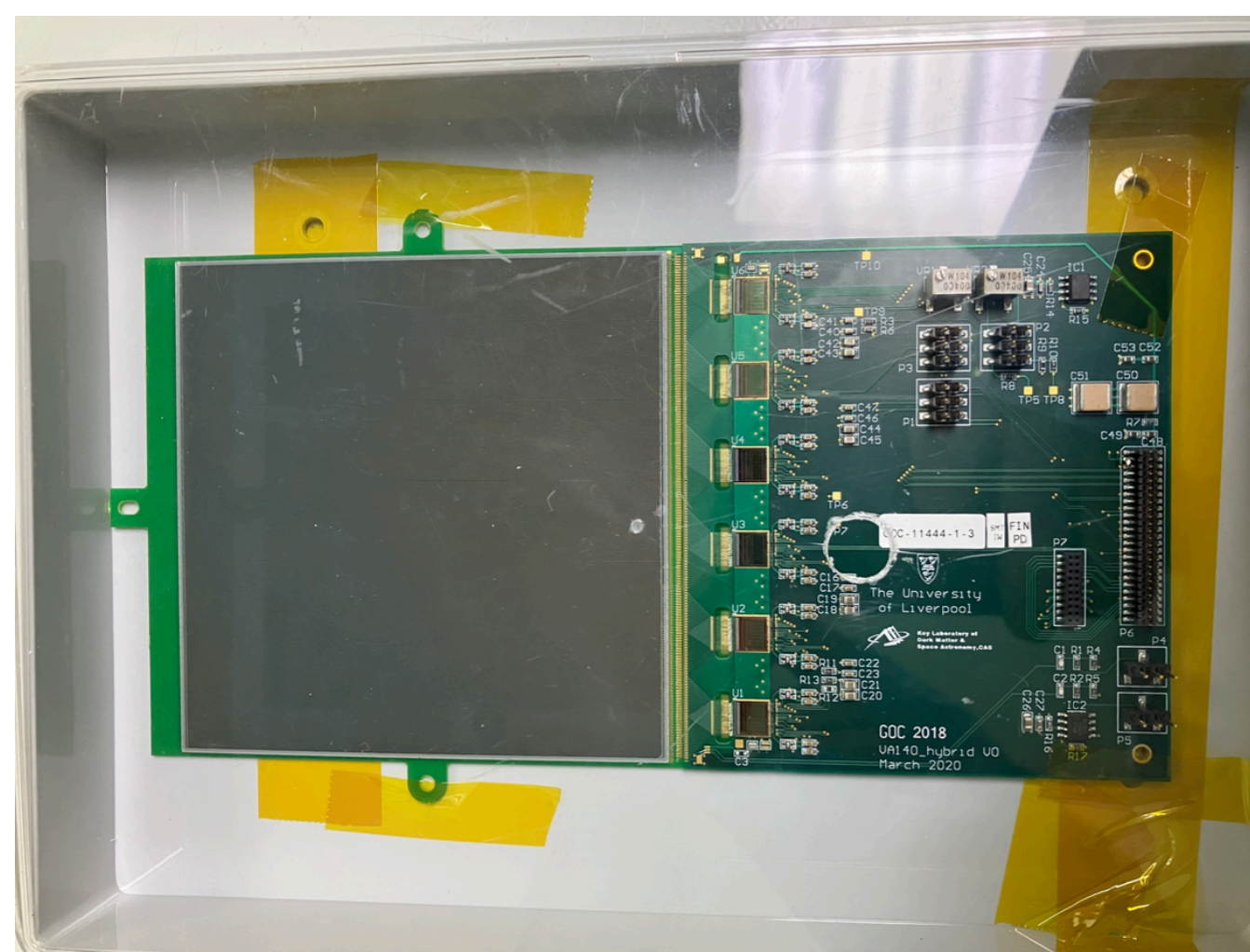
~10x10cm DAMPE sensor with VIKING ASIC
