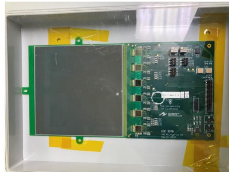
~10x10cm DAMPE sensor with VIKING ASIC
