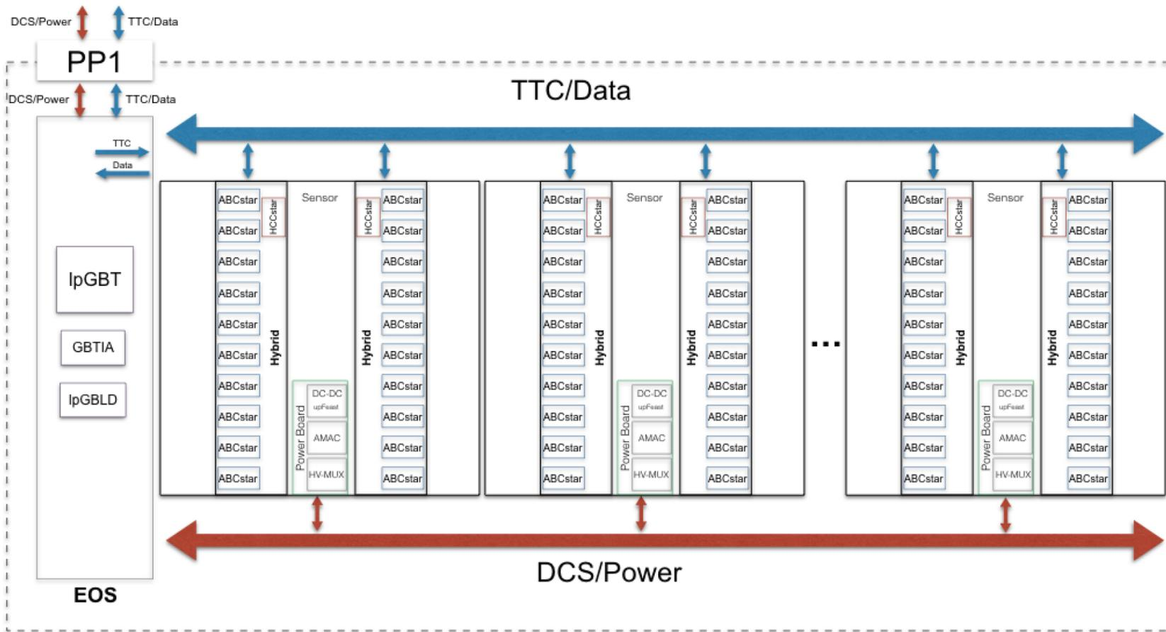
Staves and Petals have in common that DCS/Power and TTC/Data are separated to two different sides of the module.
