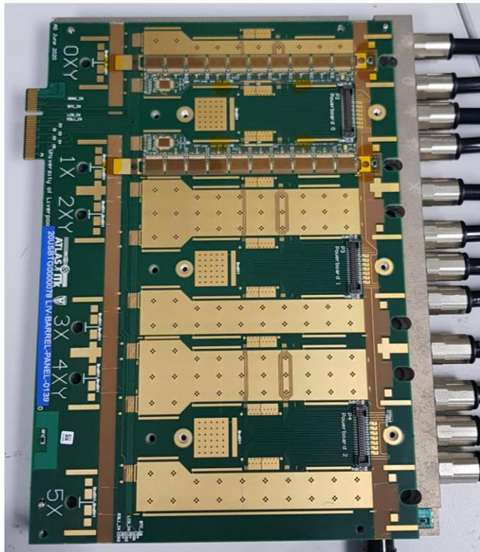
Hybrids placed on dedicated PCB for wire-bonding and electrical tests
