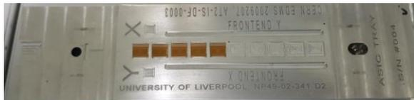
Chips placed in alignment jig with precision machined pockets to ensure correct placement of chips for gluing process
