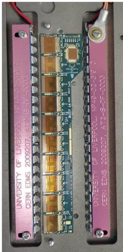
Hybrid placed back on assembly jig
