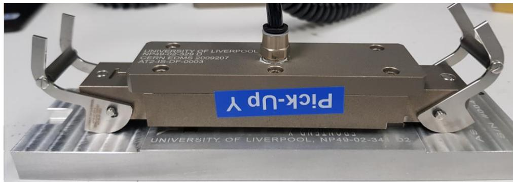
Precision vacuum tool used to pick up ASICs from alignment jig
