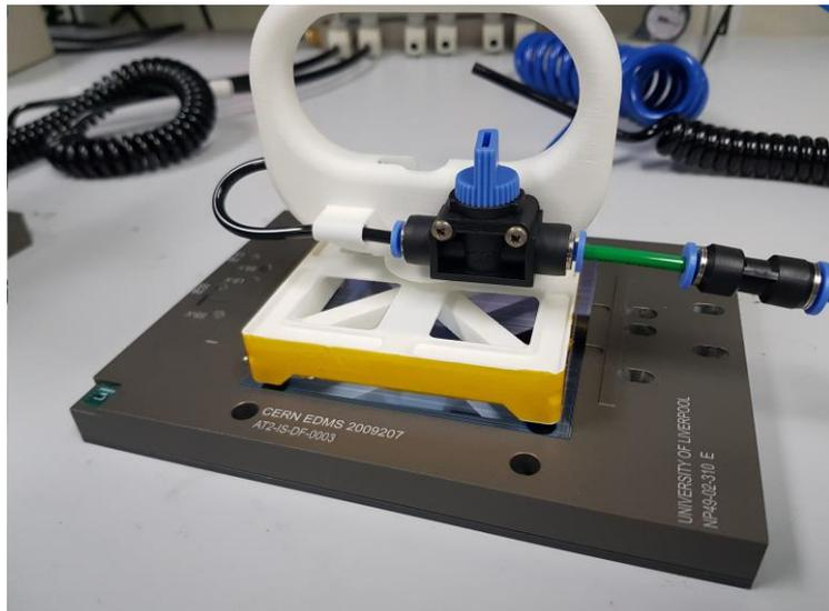
Place sensor on module assembly jig
