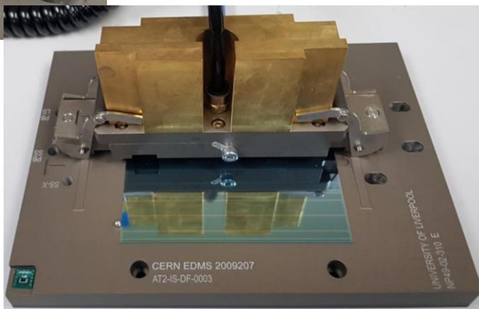
Glue needs between 4-6 h to cure enough so that the vacuum tools can be removed
