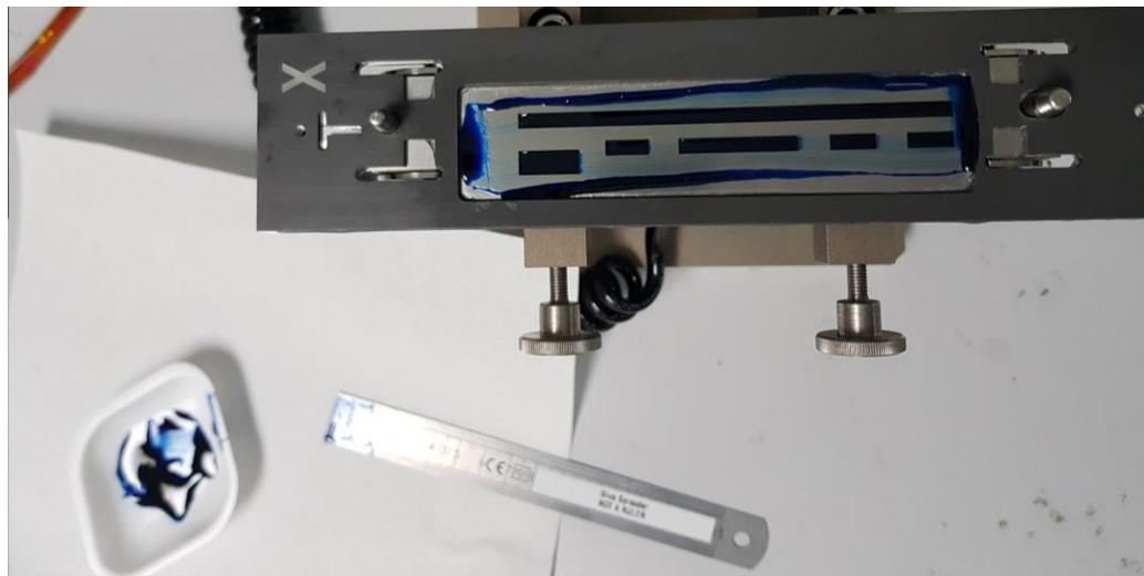
Glue for attachment of hybrids and powerboards to the sensor surface:
