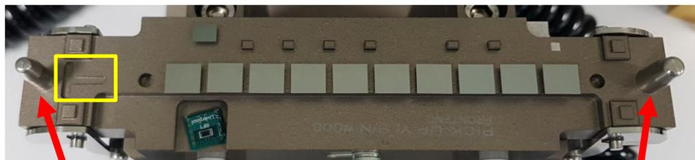
Dowel holes and pins in jigs and vacuum tool used for alignment
