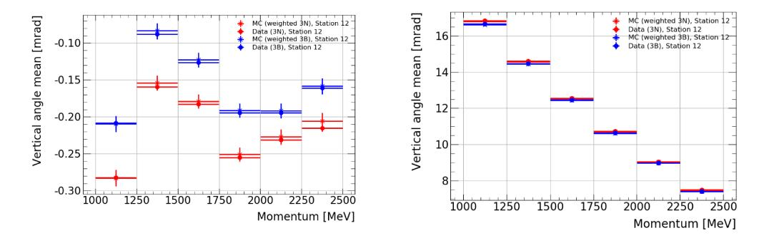
Residual differences treated as a systematic uncertainty: propagated through to the impact on the final tilt.
