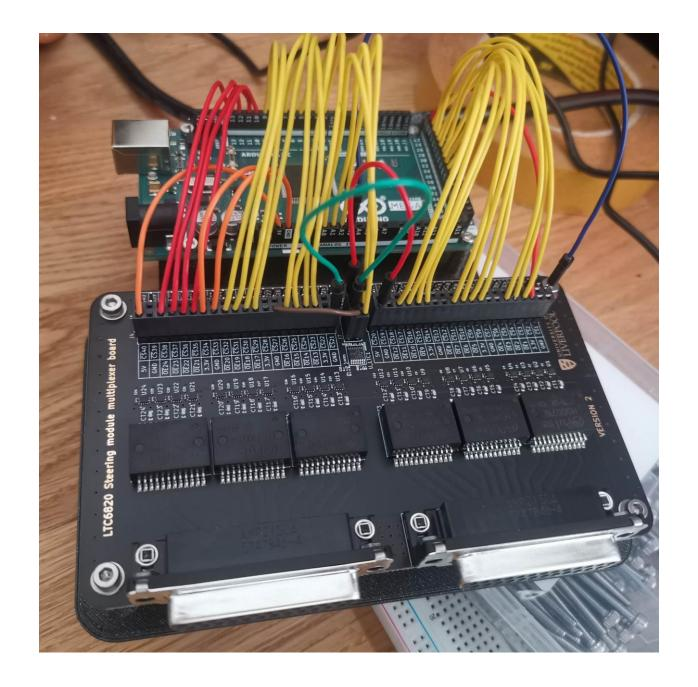
Version 2 board with new termination resistors is working.
