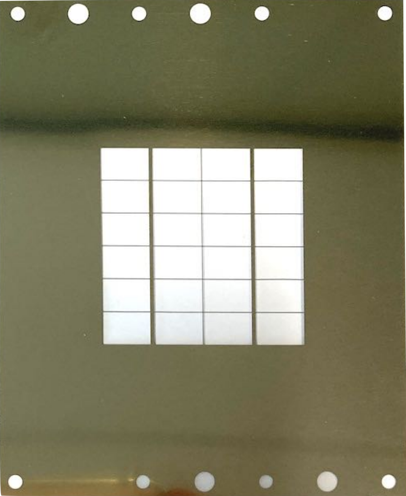
SiPM alignment stencil (chemically etched)
