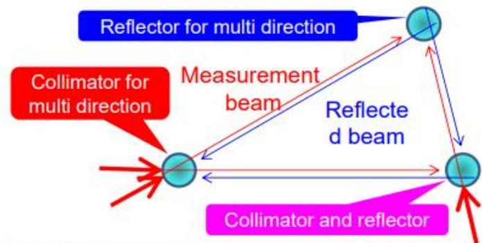
✓ Combine multi functions for the optical system of the measurement grid
