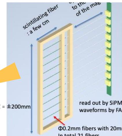
$\Phi 0.2$ mm fibers with 20mm interval. In total 21 fibers.
