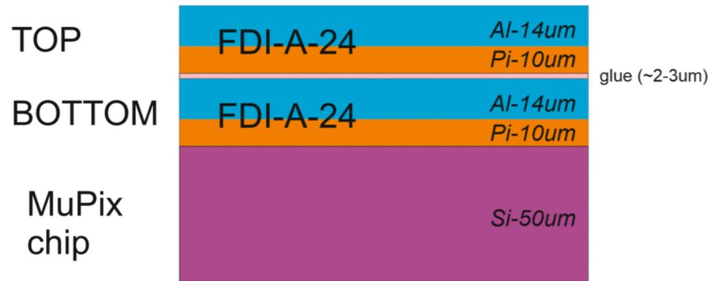
**High-Voltage Monolithic Active Pixel Sensors MuPix**
