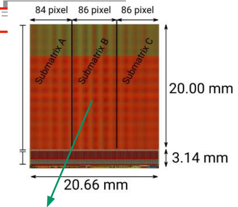
MuPIX: High Voltage Monolithic Active Pixel Sensors, pixels and the detector electronics are integrated into the same chip
