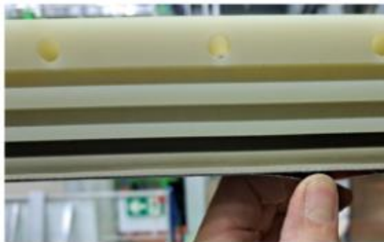
Checking grooves for o-ring and for charge labyrinth on cathode flanges
