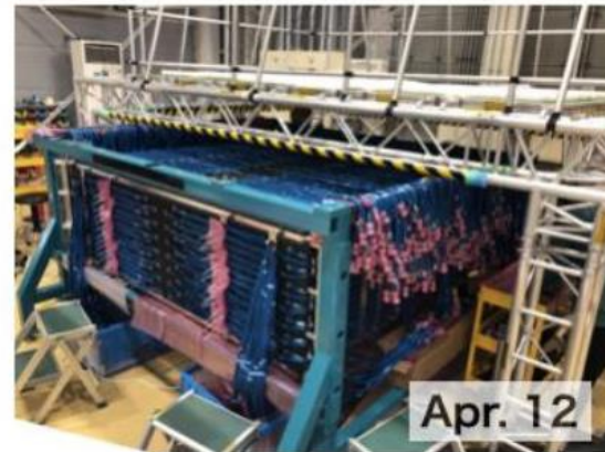
(xii) Light barrier/cables assembly
