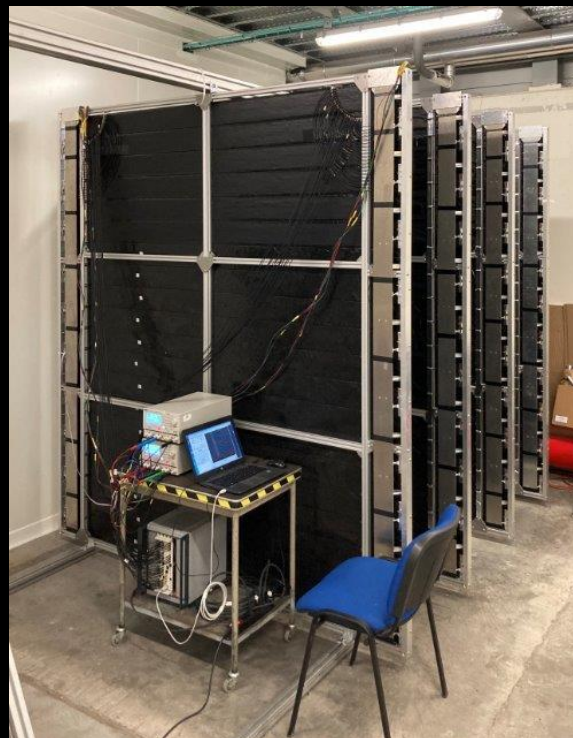
ToF modules during commissioning at CERN
