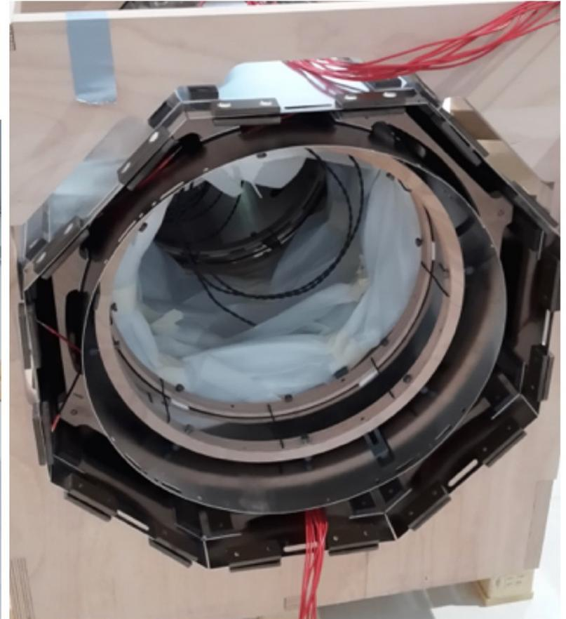
Modular design based on experience in neutron EDM and atom interferometry experiments (P. Fierlinger. TU Munich)
