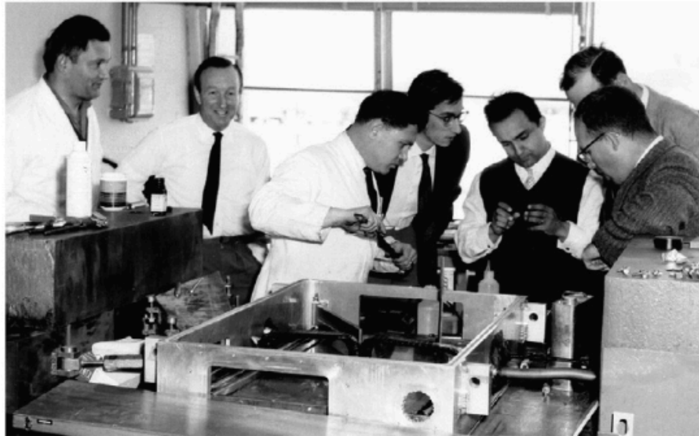
Fig. 10. The first experimental magnet in which muons were stored at CERN for up to 30 turns. Left to right: Georges Charpak, Francis Farley, Bruno Nicolai, Hans Sens, Antonio Zichichi, Carl York and Richard Garwin.
