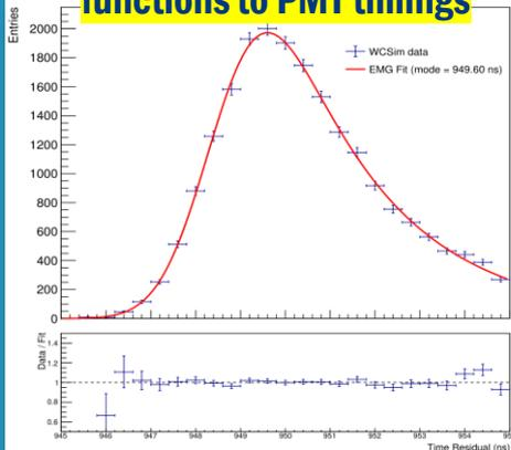
Key to calibrating against PMT timing response differences is accurately characterising the arrival time of Cherenkov photons. An exponentially modified Gaussian (EMG) function was found to be the most robust fit across varying statistics, with the mode of the distribution serving as the characteristic arrival time.
