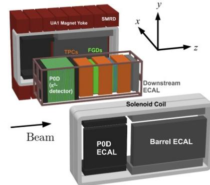
Diagram of the old ND280 near detector: composed of FGDs, TPC, SMRD, P0D, and ECAL
