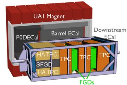
Diagram of the current ND280 near detector: composed of SFGD, FGDs, TPC, HATPC, TOF, SMRD, and ECAL
