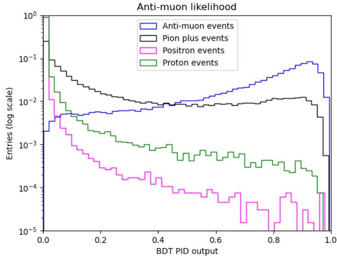
*Anti-muon likelihood: shows the likelihood of each particle type ( $\mu^+$ ,  $\pi^+$ ,  $e^+$ , and  $p^+$ ) being a muon*
