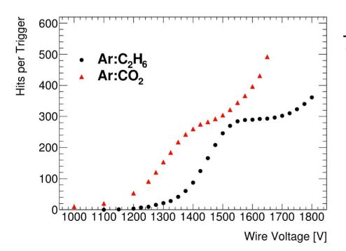
Why Ar:C2H6? → better plateau region Lower leakage rate compared to Ar:CO2 Operating voltage 1650 V in the plateau. Decided to have the best hit efficiency
