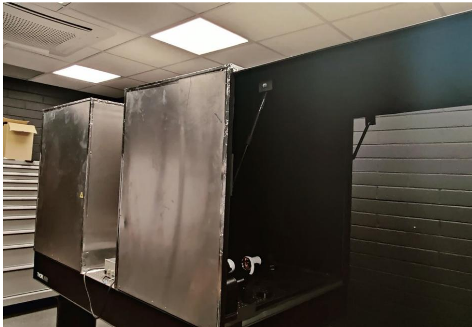
Large light-proofed dark boxes mounted on optical table
