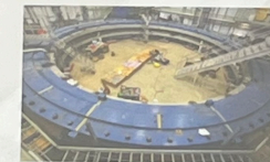
The 10-ton storage ring is being assembled in the Wilson Hall. The ring is made of 3000 segments of 10-ton segments. The fully assembled storage ring will be used to store and accelerate muons.
