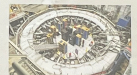
The fully assembled storage ring will be used to store and accelerate muons.
