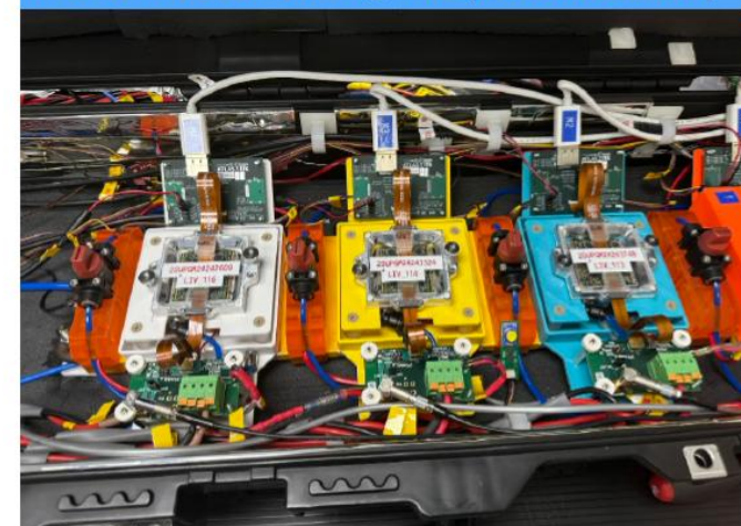
ITkPix module testing line (4x test stands)
