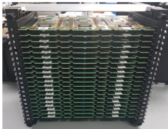
Crate with 20 hybrid panels, each holding 6 hybrids
