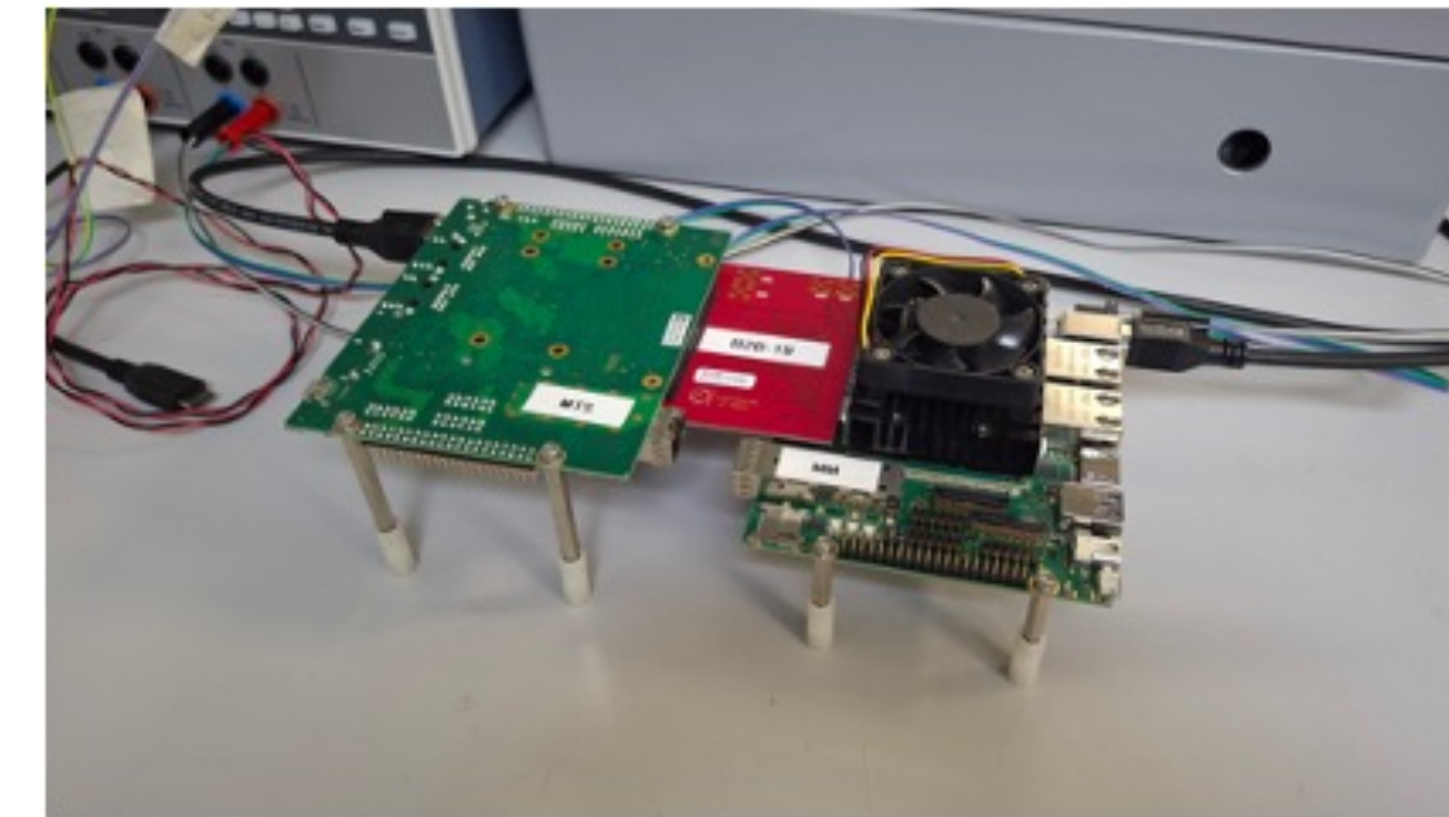
ER2: MOSAIX first ITS3 sensor prototype in LSDC
