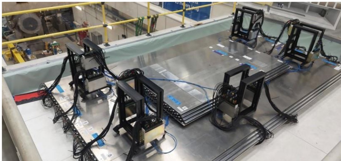
CRV installed above tracker and calorimeter
