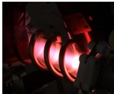
T < 1\text{eV} , L \sim \text{several cm} PF plasma (hand-made)
