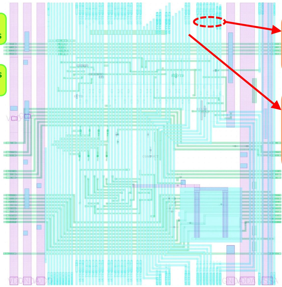
These lines are ADDR0UTB<7:0> (7 = left, 0 = right). Spacing between them is 0.32 μm.
