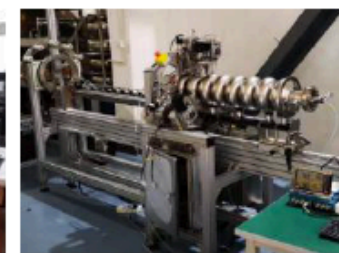
9-cell cavity pre-tuning machine
