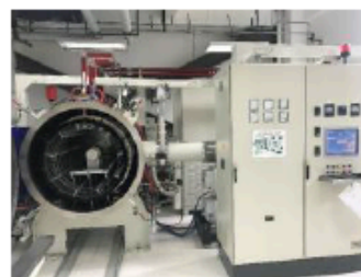
Vacuum furnace (doping & annealing)
