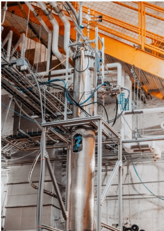
Test cryostat for circulation test Demonstrated flow rates up to 600 slpm
