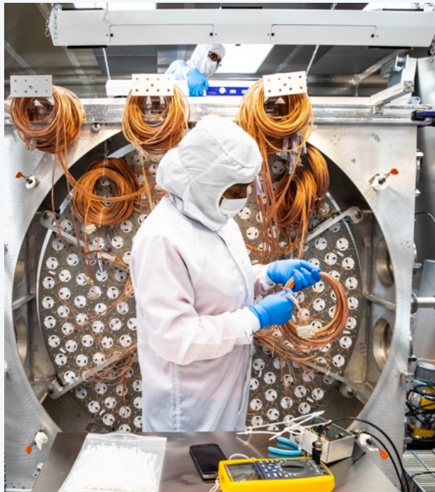
PMT array cabling at SURF
