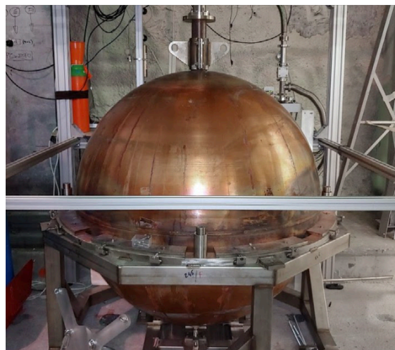
\varnothing 140 cm 4N Copper (99.99% pure) Assembled at LSM
