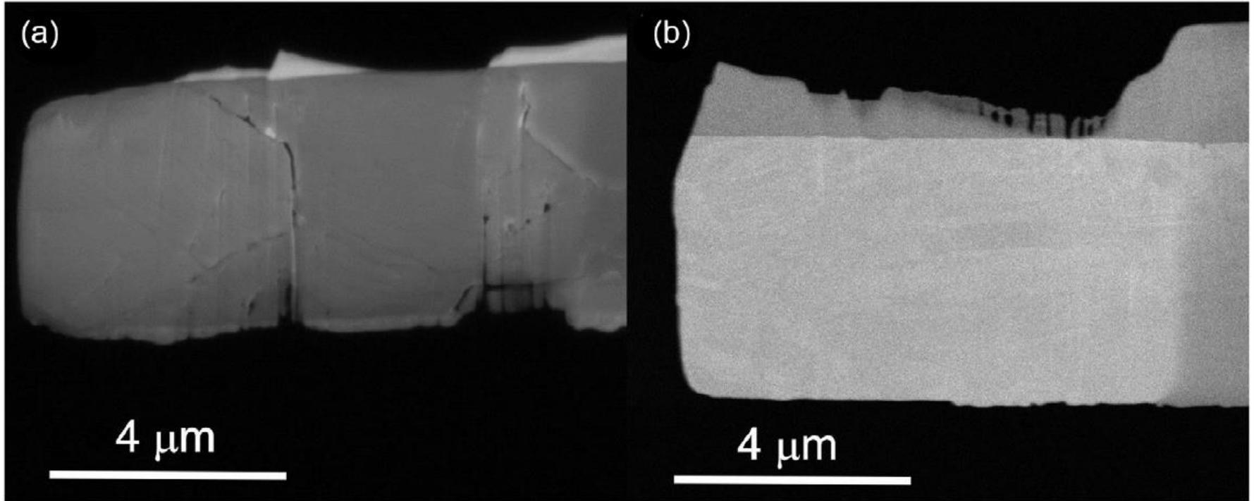
SEM images of pure (left) and Si-doped (right) B<sub>4</sub>C following 50 GPa pressure treatment
