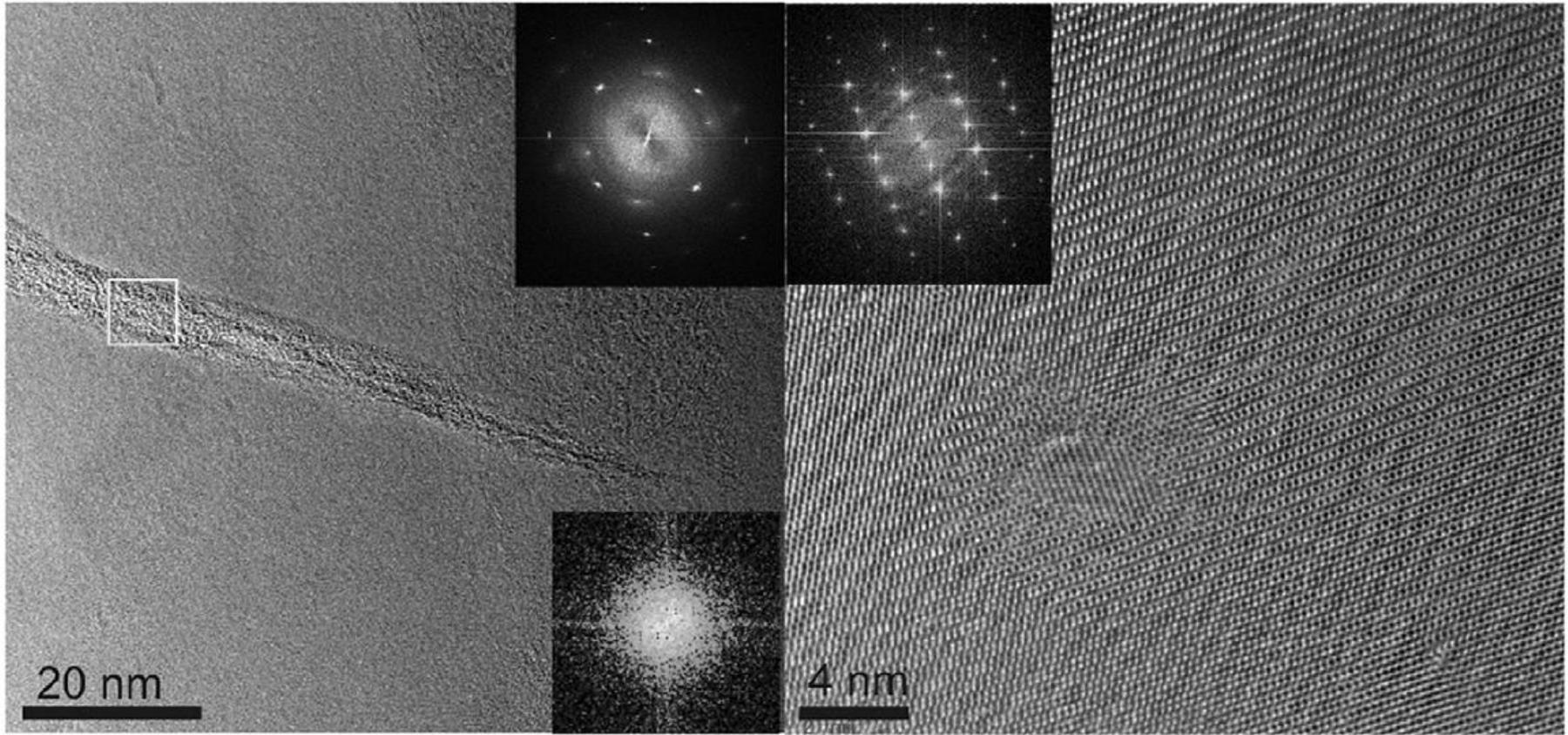
TEM images of pure (left) and Si-doped (right) B<sub>4</sub>C following 50 GPa pressure treatment
