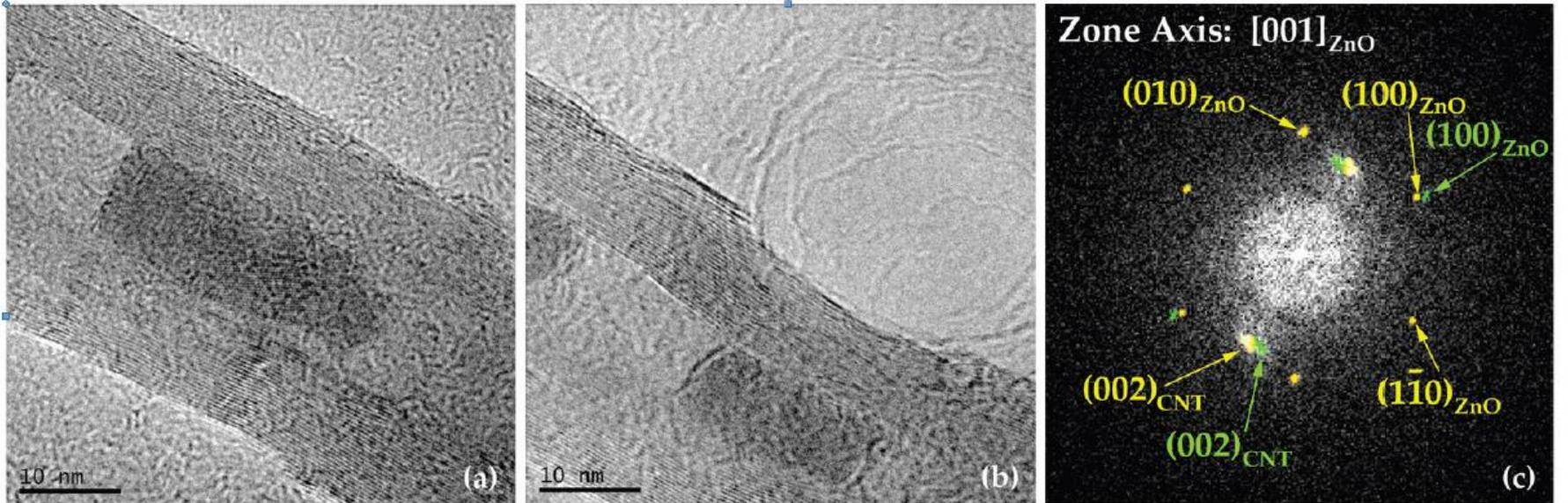
**FIGURE 8.** Radiation-induced compression of a zincite (ZnO) nanocrystal in a CNT at 500 °C. (a) The crystal prior to irradiation. (b) Same crystal after irradiation for 5 min. (c) Superimposition of FFTs from **a** in yellow and **b** in green. Compression is indicated by an approximately 6% decrease in the (100) lattice spacing. (Color online.)
