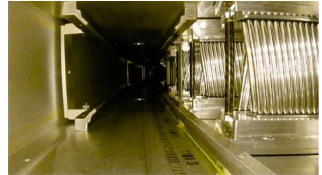
Tracking detector modules installed in the storage ring vacuum chamber
