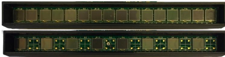
2.3x0.12 m<sup>2</sup> bars of EJ-200 PVT scintillator read out with Hamamatsu SiPM arrays
