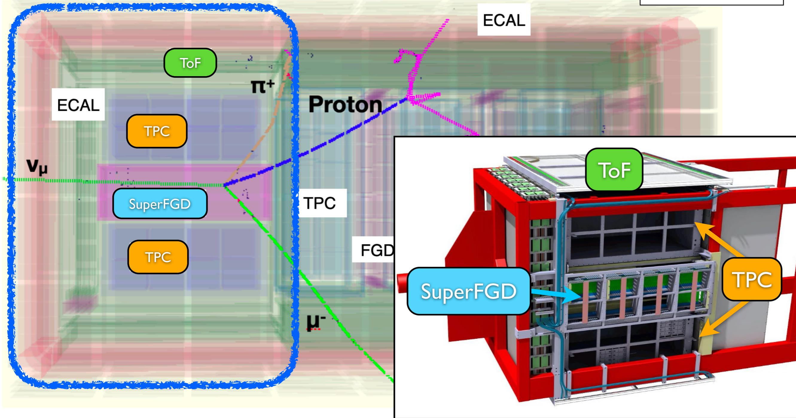
Replace part of the P0D detector (measured NC  $\pi^0$  production) with a new scintillator target (SuperFGD), two TPCs and a ToF detector
