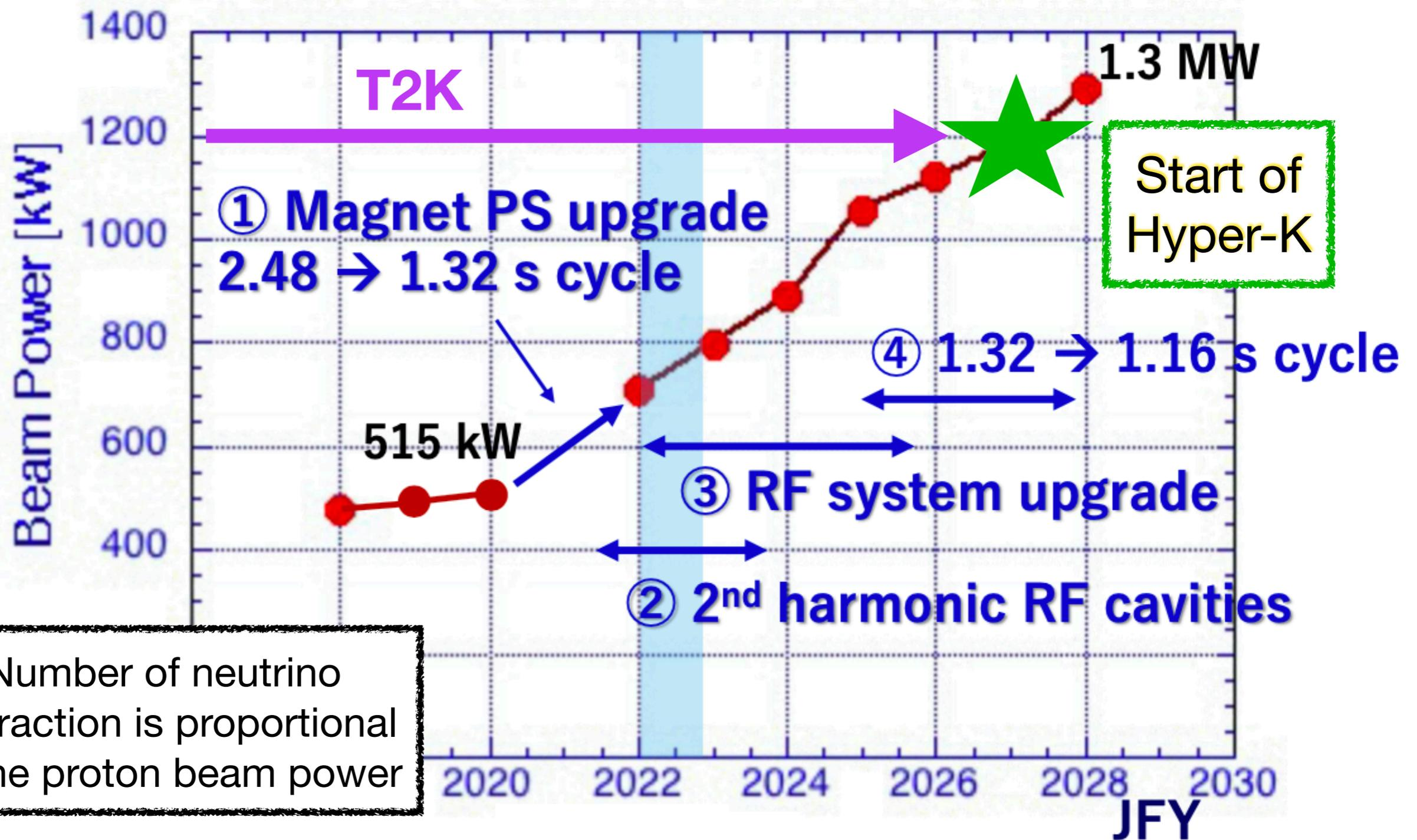
Beam power up from 515 kW to 1.2 MW at the end of T2K
