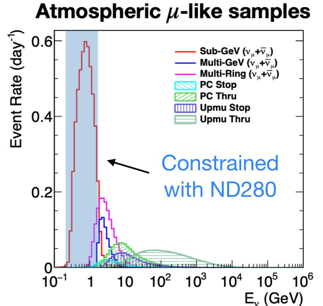
The Near Detector will constrain also cross section model of the  $\nu$  atmospheric dominant sample
