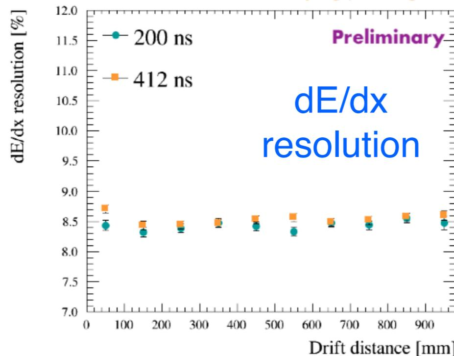
Inclined tracks with varying drift distances
