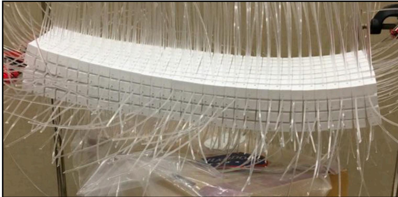
Need a method to make a unique block of plastic scintillator with all the cubes optically isolated ready just for inserting WLS fibers
