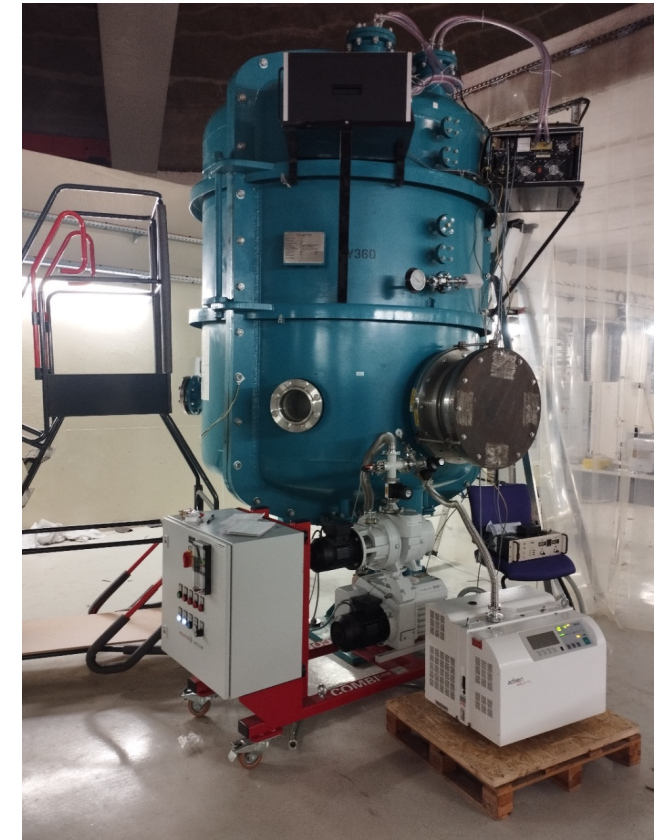
HV vessel tightness test 9/22
